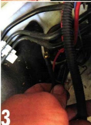
**3** Route the antenna cable neatly through the grille, along the side of the engine bay and through the firewall. Here we have been able to pass it through an existing wiring harness grommet, but if none exists, drill a hole and fit a grommet.
