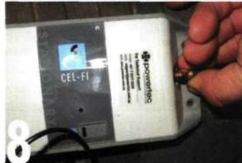
Now attach the external antenna to the unit on the port marked with the antenna symbol. If you are using an antenna supplied with the Cel-Fi GO unit, it should screw straight on to the terminal.
