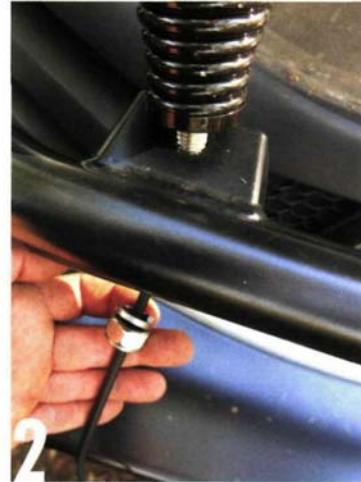
**2** While the centre of the roof or headboard is the best location for reception, it is hardly practical in reality. Most antennas will be mounted to bullbars where they are less likely to catch on low tree branches, low shed roofs or city carparks. If your bulbar does not have a mounting tab, there are plenty of bolt-on options. Choose a stainless steel one if possible. Run the cable through the hole and attach using a nut and spring washer.
