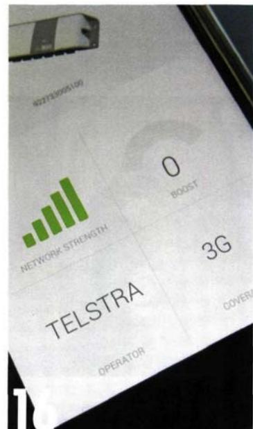
Conversely, if the network strength is high, the unit may not boost the signal at all. Low boost can also be in indication of poor antenna separation, so if both network strength and boost are reading low, adjust relative antenna placement.
