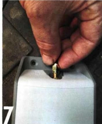
Attach the broadcast antenna to the Cel-Fi GO unit to the terminal marked with a phone symbol. Note we have left enough slack in the cables to allow the unit to be slid out from under the seat for installation and testing purposes.
