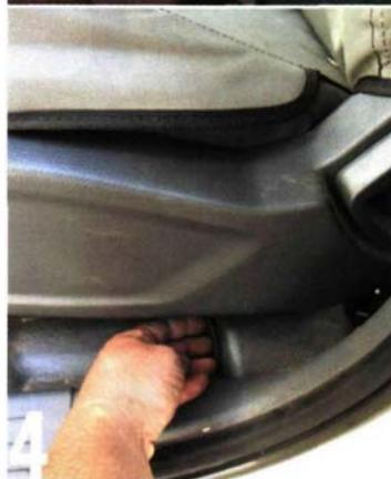
**4** As we decided to locate the Cel-Fi GO under the front passenger's seat, we have run the antenna cable under the scuff plate to the side of the seat. When choosing a location for the repeater unit, make sure it has good airflow to allow sufficient cooling. Another option is to mount it under the dash. Be sure not to interfere with airbag locations and functionality.
