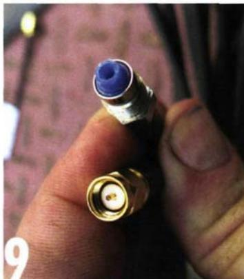
If you are using an external antenna from another supplier, it is most likely have a female FME connector (top). The exception is the supplied Blackhawk antennas which come with a male SMA connector (bottom) that matches the Cel-Fi GO SMA female connection. A male FME to male SMA adapter can be purchased for a few dollars to connect antennas from other suppliers to the Cel-Fi GO.
