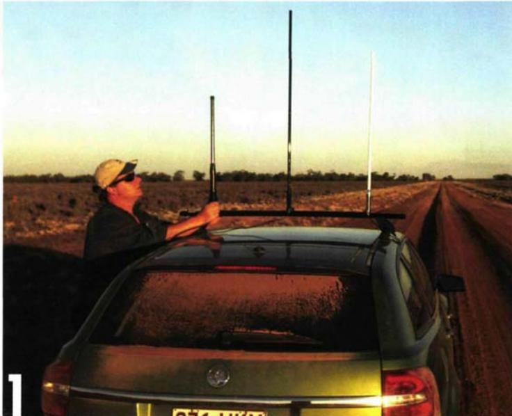
**1** The choice and position of antenna makes a massive difference to the performance of the Cel-Fi GO. In general, choose a dual band 3G/4G antennas with the highest gain possible. See our test of high gain antennas on page 34 for more information.
