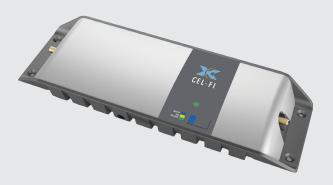
Cel-Fi GO Stationary is an evolved cellular smart signal booster design that can amplify cellular signals up to 100dB. Connect a single Donor Antenna to receive the macro-network signals, and then a single indoor Service Antenna where you need service, and Cel-Fi GO will do the rest automatically.
